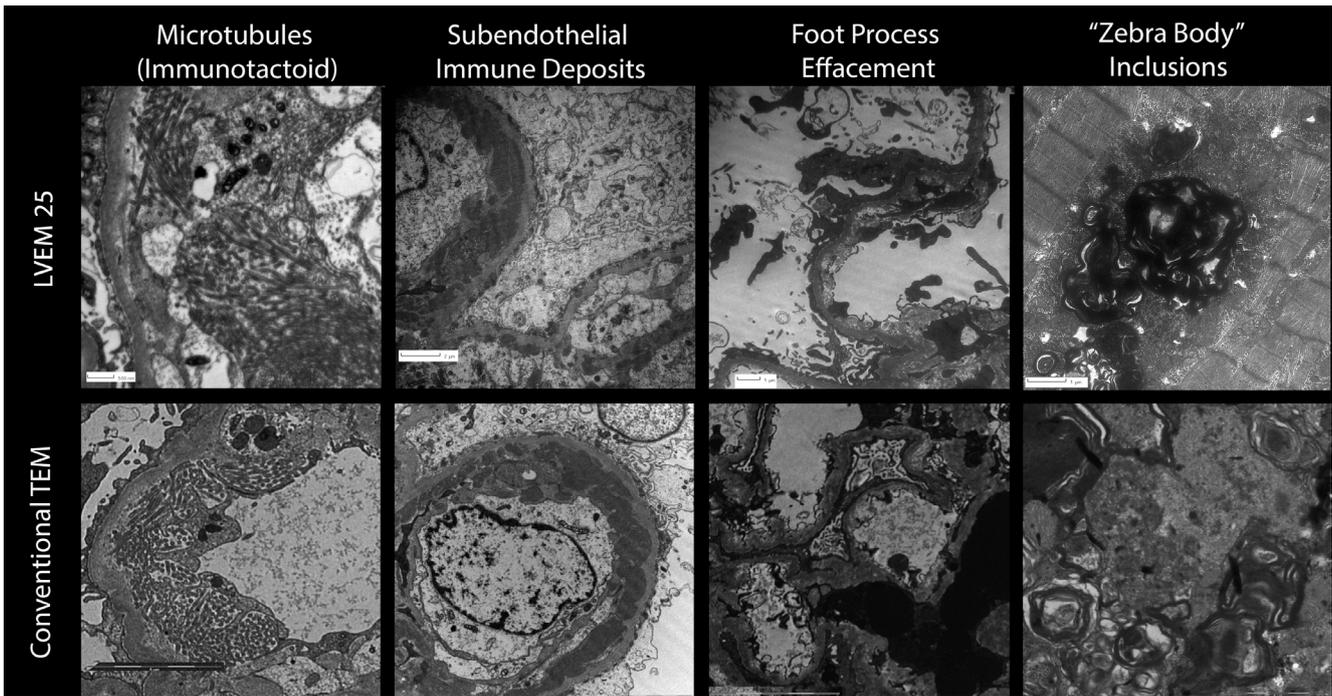
Figure 5. Side by side comparison of conventional TEM and compact LVEM images for pathology analysis. [3]
